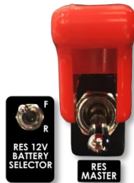
Figure 4-1 Guarded RES master switch and battery selector switch
