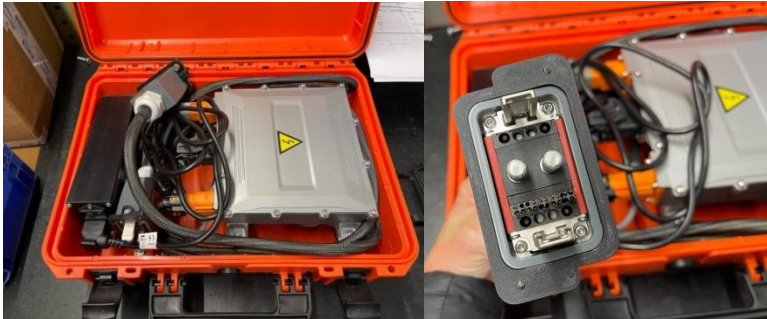
Figure 8-3 RES HV battery charger
